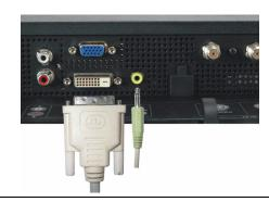
A digital signal that can support digital and convert analog to digital. DVI can be used for high resolution display and can support resolutions up to 1360 x 768.
