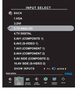
**VGA** — Select when your LCD TV display is being used as a computer monitor and you have connected the computer using a VGA cable. See "Bottom View" on page 8 for the location of the VGA connector.
