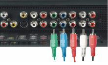
Component splits the video signal into three signals, two color and one black-and-white. To locate the connector, see "Bottom View" page 8.
